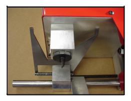
Keys are loaded into the machine with the tip at the right and the head of the key to the left. Secure the key in the vise with the Vise Lock Nut (T-Nut); snug the key into place but do not over tighten the lock nut.
