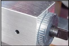
The depth guide on the MD-1 is adjustable in the event the machine ever needs calibration.
