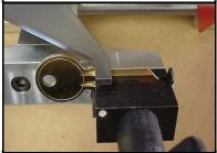
The key vise used on the MD-1 has two sides. The side of the vise with the small dot is the narrow side of the vise, used when cutting most single sided keys that have deep cuts. The wide side of the vise will hold most double sided keys without tipping. The depth of cut on either side of the vise will be within .001".
