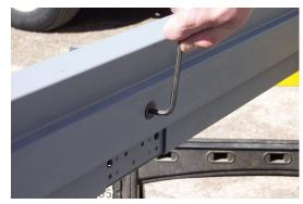
The tool is double-sided; after extensive use some wear may be evident in the threads or face of the tool; simply use the opposite side. Two allen screws and a long-arm allen wrench are also included.
